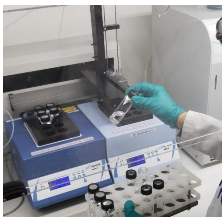
SD-1BM blocks with an optional chiller
